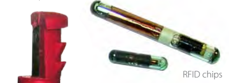
Plastic fastening encapsulating RFID chips
